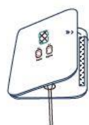
Step 4: Peel off the adhesive, fold the left side over, and wait for 15 minutes.
